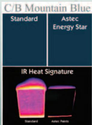
As a result of ongoing research and development into heat reflective coatings Astec developed a new technology of colour infused nano ceramics that reflect heat by selective reflection of infrared light. This technology has enabled us to offer dark colour exterior coatings that reflect fully 50% of Solar energy and provide positive results for our environment and consumers.
