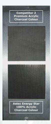
All four samples were identical in colour at the beginning of the test cycle. At the end of the test cycle all premium acrylics had chalked and lost their original depth of colour. Whereas the Astec Energy Star acrylic retained it's gloss, mechanical properties and original depth of colour.
